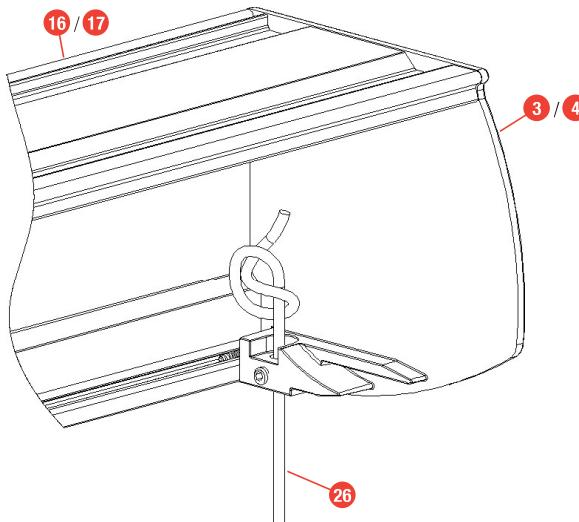
**(GB)** Wall assembly system of the UNIVERSAL SCREEN with Rope.
